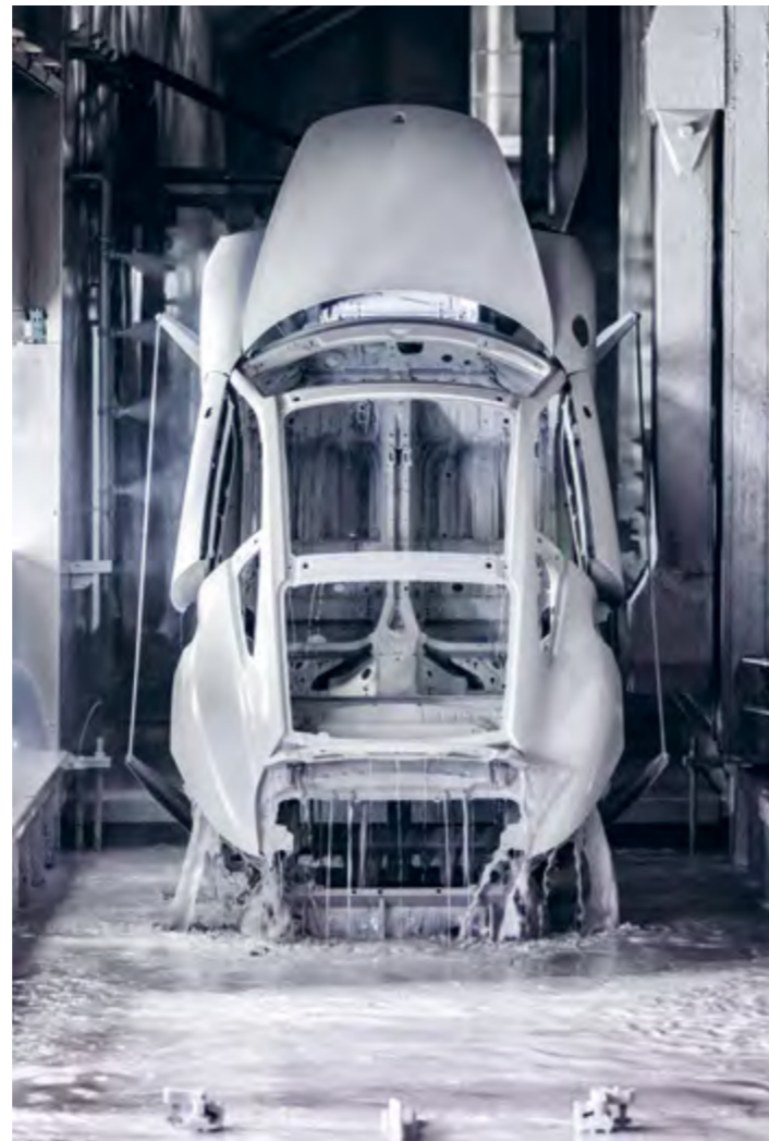
PRODUCTION IN ZUFFENHAUSEN: CATHODIC DIP COATING
